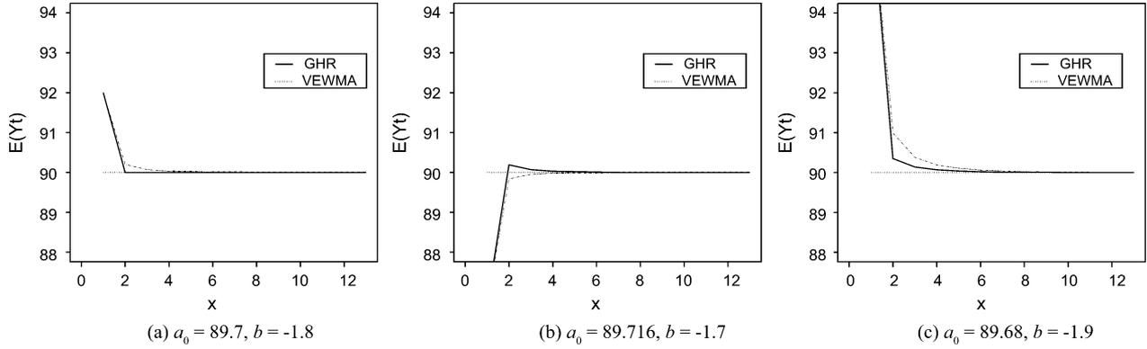
Fig. 9. Mean responses of a process controlled by GHR and VEWMA controllers when initial bias exists.
