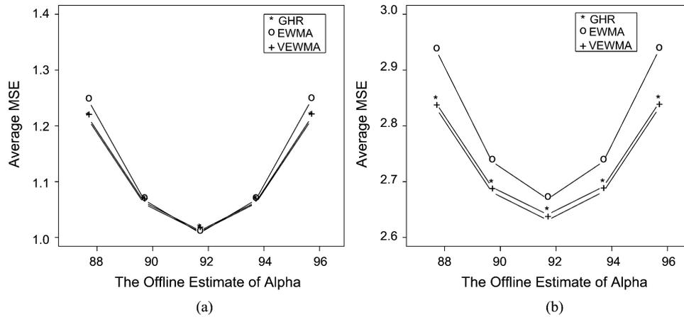
Fig. 4. AMSE of the EWMA and GHR Controllers when  $N_t$  is an ARIMA(1,1,1) process but is misidentified as an IMA(1,1) process. (a) ARIMA with  $\phi = 0.2$  and  $\theta = 0.6$ . (b) ARIMA with  $\phi = 0.6$  and  $\theta = 0.2$ .
