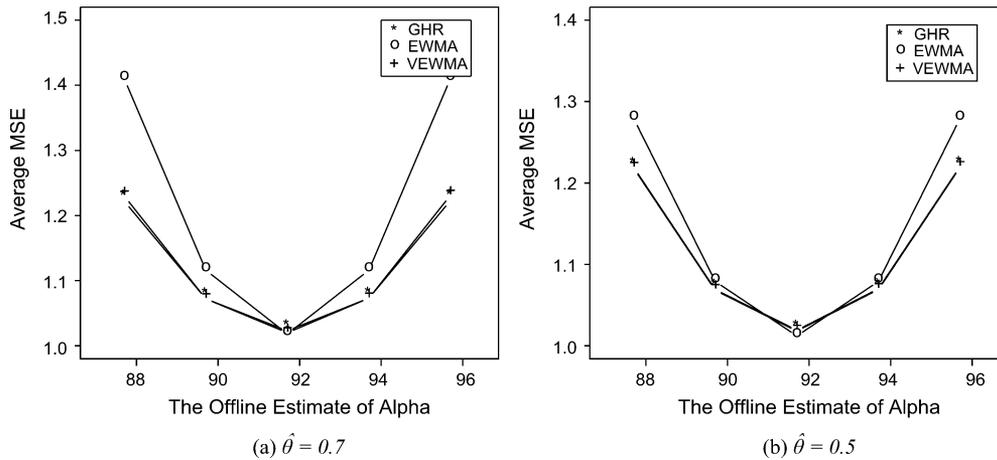
Fig. 3. AMSE of the EWMA and GHR Controllers when  $\theta$  is Over- and Under-estimated.
