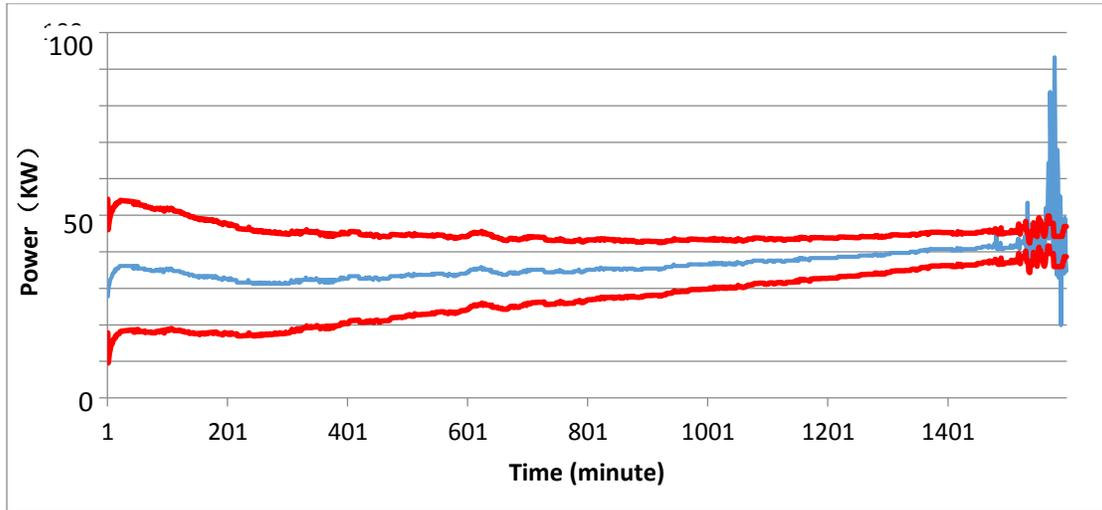
Figure 8. Control chart for the power curve of an abnormal ingot
