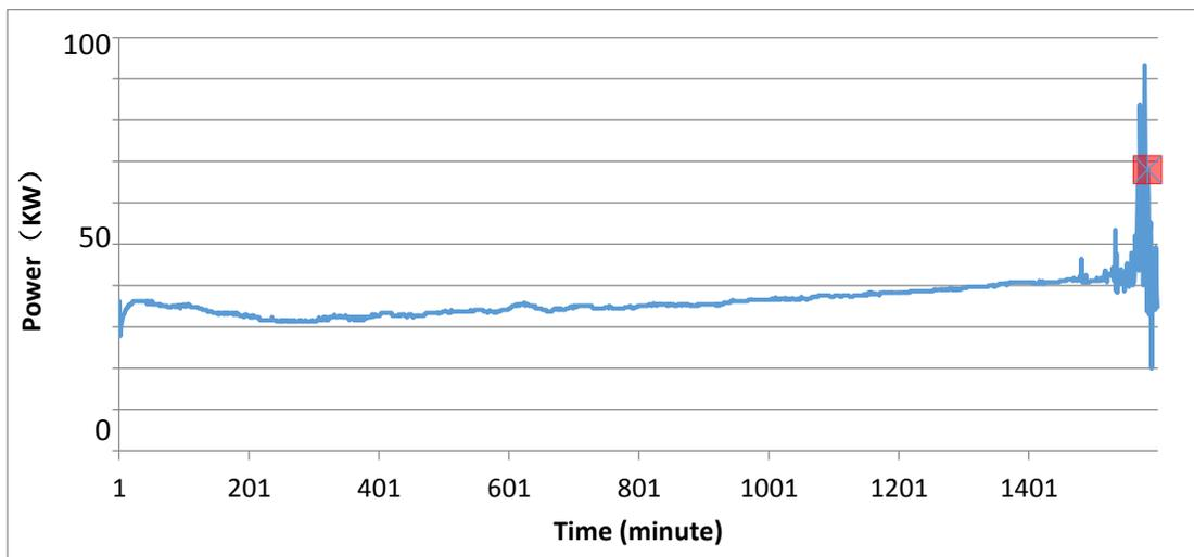
Figure 4 Time series plot of power in an abnormal run
