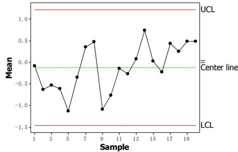
Figure 1. A typical control chart with constant mean and variance
